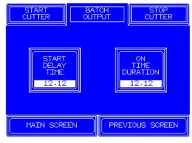
Outputs 1, 2, 3, Pre-Batch and Batch are 24VDC sinking digital outputs with a max. load of 100 MA. For wiring refer to cutter schematic. The outputs turn on every time the knife cycles one cut.
