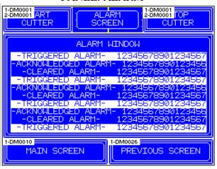
• To delete an alarm, press in the middle of the screen. A menu will appear at the bottom of the screen. Press MODE. Press DELETE. Press DONE. Exit Alarms. *NOTE:* When machine is powered down all ALARMS are lost. There is no memory for past alarms.
