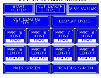
• **DISPLAY UNITS** - Press the DISPLAY UNITS button. The cut length units screen will appear. Cut length units changes the count to inches, feet or (optional) centimeters and millimeters. *NOTE*: When changing units, the controller automatically will convert all part lengths to the newly chosen unity type.
