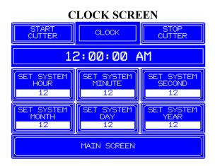
*NOTE*: To adjust the contrast of the screen, simultaneously touch both upper screen corners. A contrast bar will appear on the bottom of the screen. Press the desired setting then press anywhere on the screen to remove the contrast bar.
