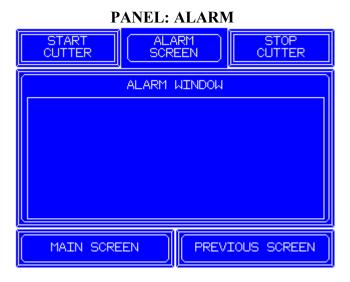
• To delete an alarm, press in the middle of the screen. A menu will appear at the bottom of the screen. Press MODE. Press DELETE. Press DONE. Exit Alarms. *NOTE:* When machine is powered down all ALARMS are lost. There is no memory for past alarms.
