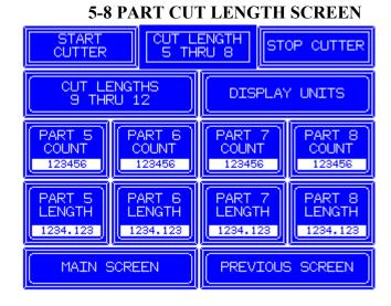
• **DISPLAY UNITS** - Press the DISPLAY UNITS button. The cut length units screen will appear. A cut length unit changes the count to inches, feet or (optional) centimeters and millimeters. *NOTE*: When changing units, the controller automatically will convert all part lengths to the newly chosen unity type.
